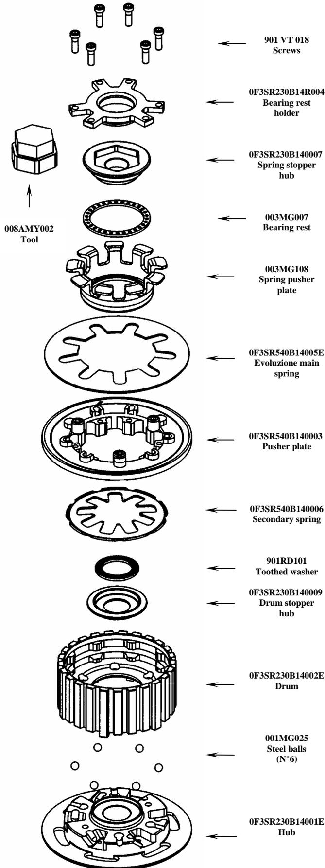
Perform the assembly starting from the hub pack: put the hub (0F3SR230B14001E), put the 6 steel balls (001MG025), at the bottom of grooves using a little bit of grease.
